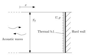
**Figure 4.6** – Schematic of a hard acoustic wall where the thermal boundary layer dissipates a bit of the acoustic energy ( $Z \neq \infty$ ).
