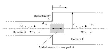
**Figure B.1** – Schematic of a discontinuity at the interface between two tubes with different radius. Domain B is the smaller tube and domain C is the larger tube. The radius of the tube in domain B is b, and the radius of the tube in domain C is c.
