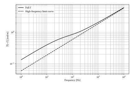
**Figure 4.2** – Logarithmic plot of the negative of imaginary part of the viscothermal wave number  $(-\Im [\Gamma])$ , for a tube with a diameter of 1 mm. In blue, the full  $f_{\nu}$  and  $f_{\kappa}$  of Eq. 4.16 and 4.3 is used. The orange curve corresponds to Eq. 4.18.
