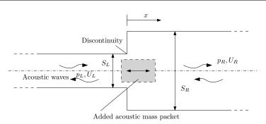
Figure 4.4 - Schematic of a waveguide discontinuity.
