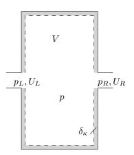
Figure 4.3 - Schematic of the compliance volume segment.
