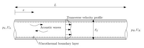
Figure 4.1 – Geometry of the prismatic duct
