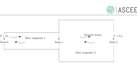
Figure 3.1 - Example of two simple duct segments connected together.
