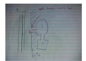
**Figure 4.7** – Schematic view of incident wave (green) on an infinite wall (blue) containing a port with a system connected to it. The location of the boundary condition is shown in red.
