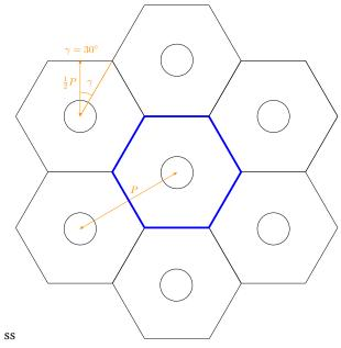
Figure 7.1 – Geometry details of a hexagonal hole pattern
