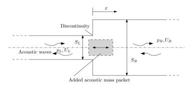
Figure 4.4 - Schematic of a waveguide discontinuity.
