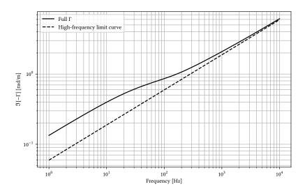
**Figure 4.2** – Logarithmic plot of the negative of imaginary part of the viscothermal wave number  $(-\Im[\Gamma])$ , for a tube with a diameter of 1 mm. In blue, the full  $f_V$  and  $f_K$  of Eq. 4.16 and 4.3 is used. The orange curve corresponds to Eq. 4.18.
