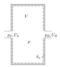
Figure 4.3 - Schematic of the compliance volume segment.
