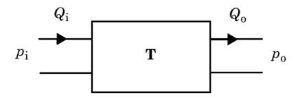
$$\left\{\begin{array}{c} p_i \\ Q_i \end{array}\right\} = \left[\begin{array}{c} T_{11} & T_{12} \\ T_{21} & T_{22} \end{array}\right] \left\{\begin{array}{c} p_o \\ Q_o \end{array}\right\}, \tag{9.1}$$
