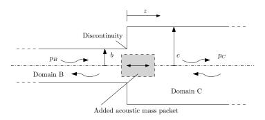
**Figure B.1** – Schematic of a discontinuity at the interface between two tubes with different radius. Domain B is the smaller tube and domain C is the larger tube. The radius of the tube in domain B is b, and the radius of the tube in domain C is c.
