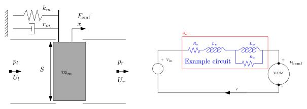
Figure 5.1 – Electrical and mechanical model of the speaker
