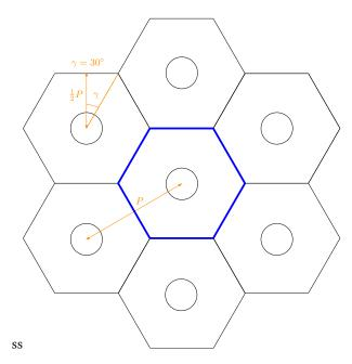
Figure 7.1 – Geometry details of a hexagonal hole pattern
