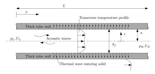
**Figure A.1** – Schematic situation of a tube surrounded by a thick solid. Note that the transverse acoustic temperature is drawn to be not zero at the wall. This happens in case of thermal interaction with a solid with finite thermal effusivity.
